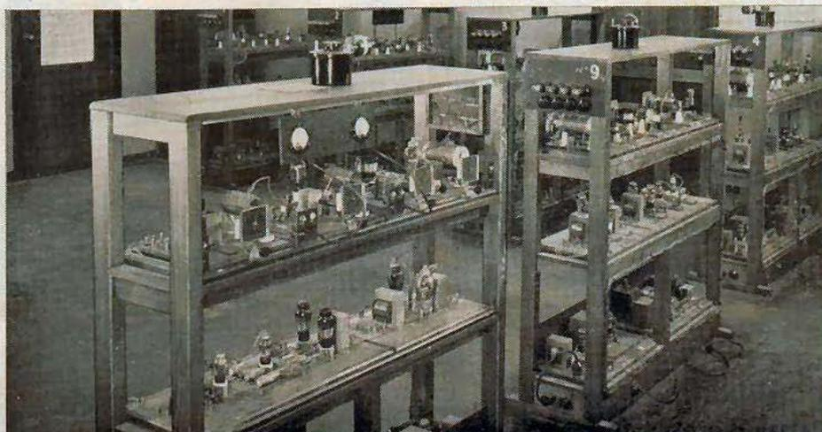
Transmitter Laboratory showing some of 10 similar open wiring type of C.W., I.C.W. and phone transmitter units.
